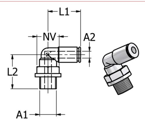
Ext. hose diameter A2 = 6L1 = 21 L2 = 14.5 NV = 9 Thread A1 = M5
